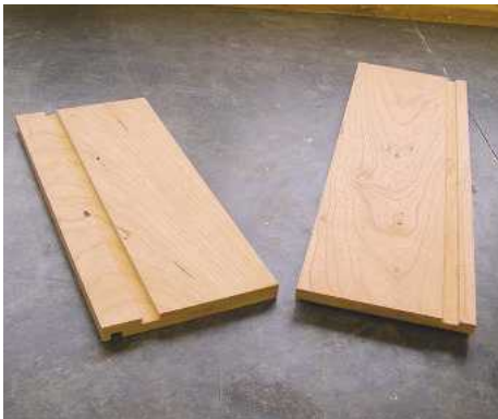
▲ Pic.16 The drawer side and front panels were routed for the drawer runners, the MDF bottom panels, and the glass inlay
